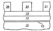
optical assist layer 16 and does not form a resist 'foot' under the resist patterns 24. A thickness of the optical assists layer 16 is optimized so as to reduce/remove interference between the resist layer and a substrate 10, and accordingly the resist 'foot' is reduced/ removed.
